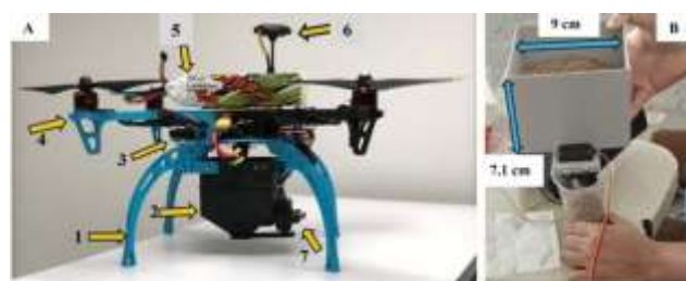
Fig. 8 A) Photograph of the constructed drone, 1) landing gear, 2) hopper, 3) main platform and controller, 4) rotor arm, 5) battery, 6) antenna, 7) seed-release mechanism. B) Picture of the designed hopper.
