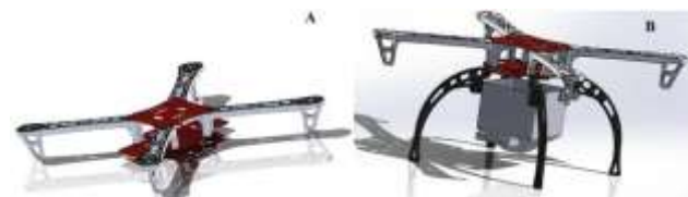
Fig. 5 CAD design of the seed-dispersal drone. A) Main platform B) Assembly of the platform and the dispersal hopper.
